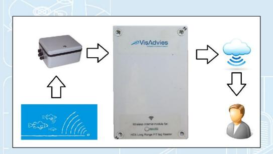
The Wireless Internet Module (WIM) for the Oregon PIT Readers facilitates data transfer from the study site to your office over the Internet in a fully automated way. The data is transferred on daily basis through a 3/4G Internet connection or a LAN network if available at the study site.
